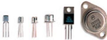
Individual Transistors (About the size of your fingertip)
