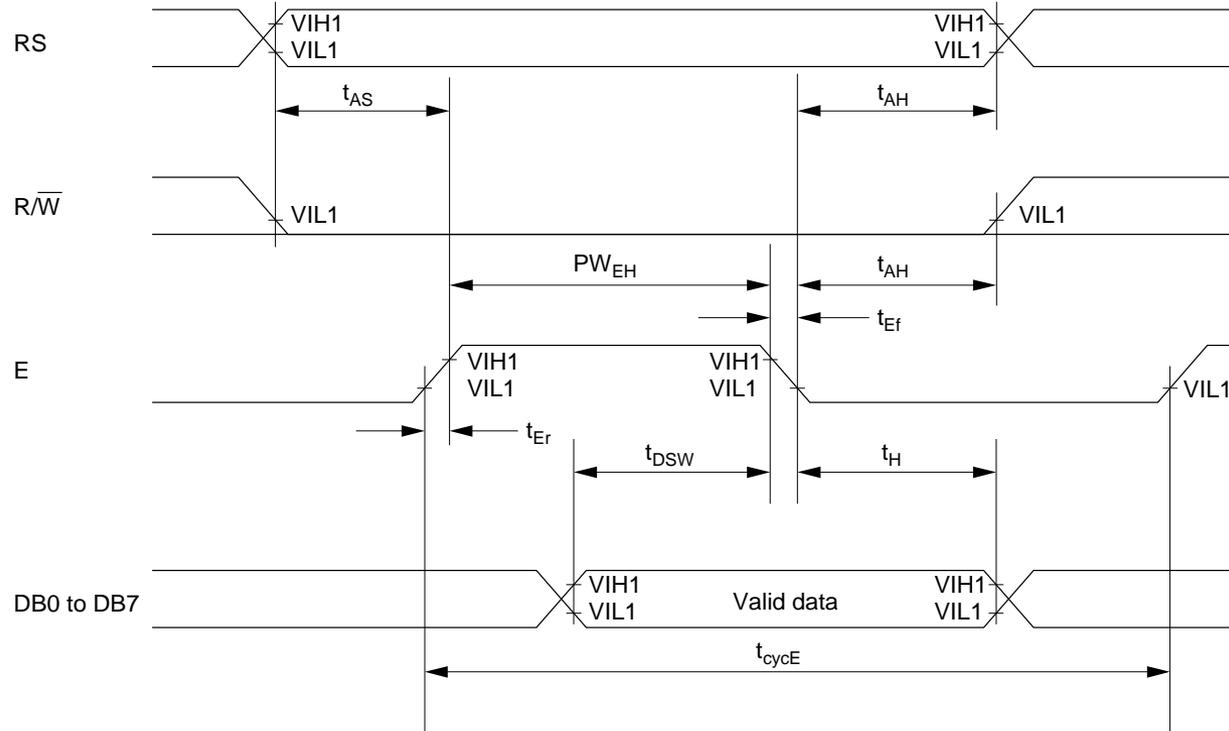
Figure 27 Write Operation
