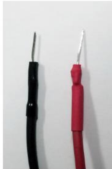
Figure 5: Test leads with pins on ends
