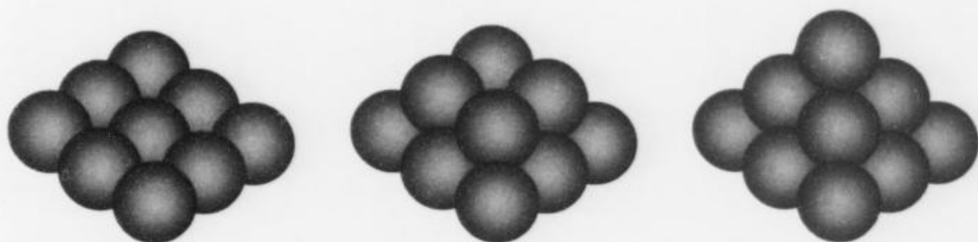
Figure 1. The way of stacking cannon balls or oranges; used in practice since we can remember, suggested as optimal by Kepler in 1611 and finally proven so by Hales in 1998.
