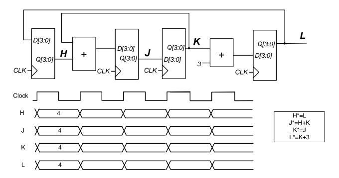
2. Complete the waveform for the sequential circuit shown below by filling in the decimal value that each register will output during each clock cycle.
