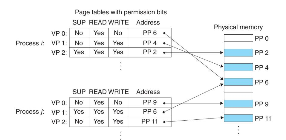
Page-level memory protection and sharing (page tables in kernel memory). Process context switch: load PTBR from GDT into CR3 register, flush TLB.
